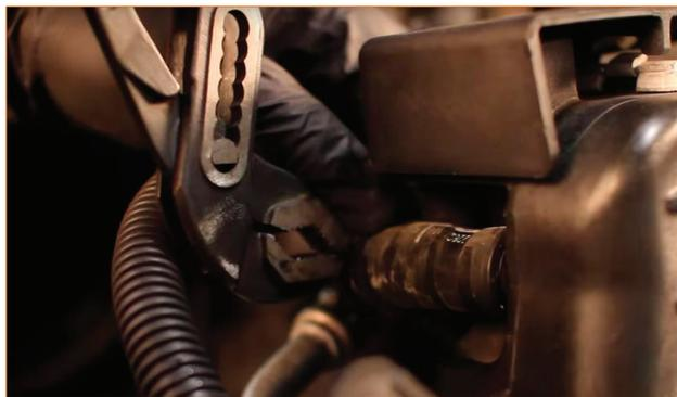
11. Remove the three tree-clips that secure the battery cable to the upper fan shroud. (3x tree-clips)
