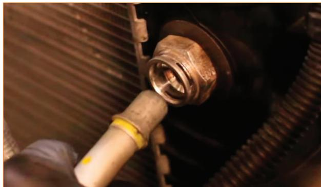
20. Remove the four bolts that secure the radiator to the intercooler. (4x 13mm bolts)
