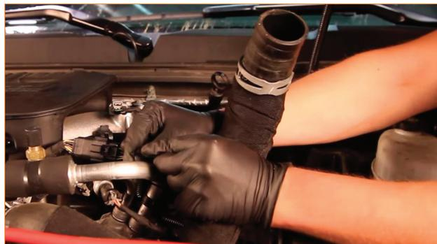
10. Remove the coolant overflow hose from the radiator, and tuck it out of the way.
