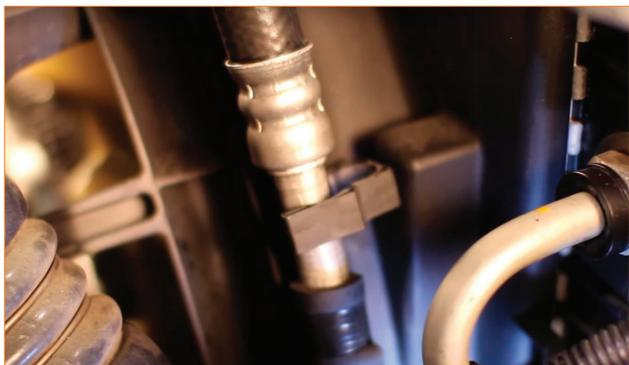
15. Remove the upper fan shroud by lifting it straight up.
