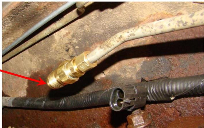
6A-6. Run the fuel line along the frame as mentioned in step 5-3 to the “Engine” port in the AirDog®. Cut the fuel line to length and insert fuel line end FQC12S per step 5-1. Once the connector is installed, connect it to the male J2044 fitting in the “Engine” port in the AirDog®. A “click” will be heard once properly connected. The finished Fuel Supply Line should look similar to figure 22.
