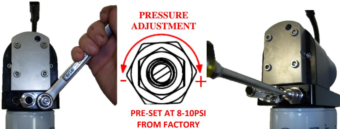
Turn the adjuster screw counter-clockwise to reduce the output pressure or clockwise to increase the pressure. Be sure to re-torque the jam nut after adjusting the regulator. **IT IS STRONGLY RECOMMENDED TO ADJUST THE PRESSURE WHILE USING A FUEL PRESSURE GAUGE. TOO MUCH OR TOO LITTLE PRESSURE MAY CAUSE DAMAGE TO THE INJECTION SYSTEM!**
