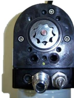
**STEP 3:** Remove and clean the Gerotor. Be very careful to not damage the Gerotor.
