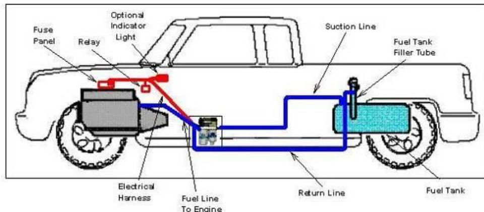
The AirDog®II-4G draws fuel from the fuel tank at a constant flow, removing water, particulates, and air/vapor. A regulated pressurized flow is maintained to meet the engine's varying fuel demands. The separated air/vapor and excess fuel not needed by the engine are returned from the AirDog® to the fuel tank.
