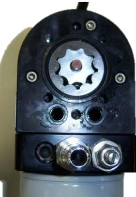
**STEP 8:** Loosen the cap screws. Torque the cap screws in an opposing pattern.
