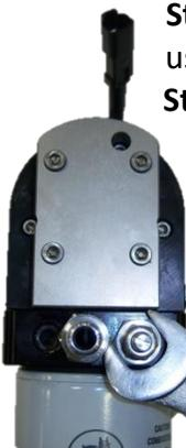
**Step 1.** Remove the regulator by turning the Adjustment Screw counter-clockwise using a 3/4 wrench.
