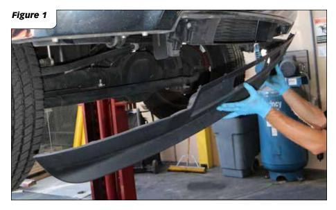
**1.** On the 2013-up Ram 2500 and 3500, the Intercooler is located behind the front bumper, underneath the radiator. To begin, remove the front bumper air dam. This requires removing the two bolts and 15 retainer clips that attach the air dam to the bumper. These can be accessed from the back of the bumper. This requires a 10mm wrench or socket and a body clip removal tool. **Figure 1**
